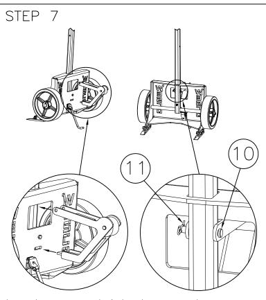
secure with clevis pin(10) and
