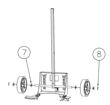
Secure wheels using four washers(7) and two cotter pins(8).
