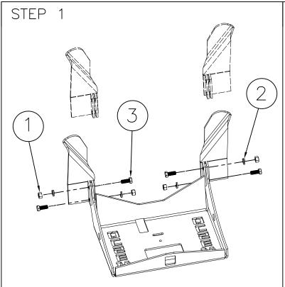
Fasten right and left toes to base using four nuts(1), four lockwashers(2), and four bolts(3). Tighten securely.
