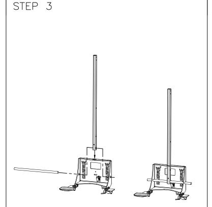
Insert axle through one axle hole in base, through post, and through opposite base axle hole.
