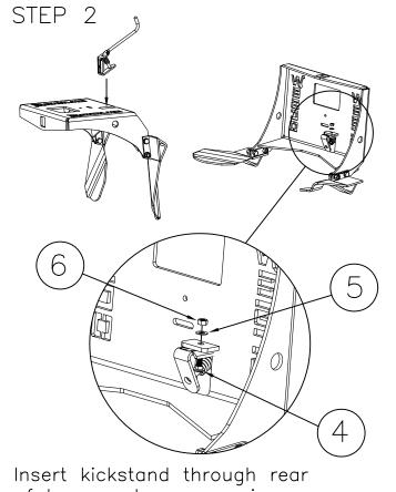
Insert kickstand through rear of base and secure using one bolt(4), one washer(5), and one nut(6).
