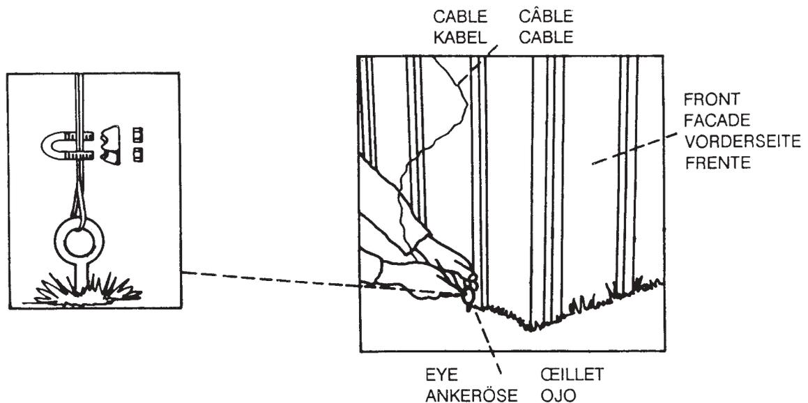
B. Insert opposite end of cable through eye, cut off leaving 4" to 6" of cable. Assemble cable clamp as shown.
