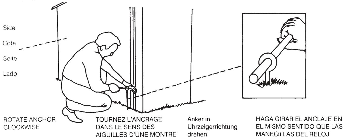
NOTE: IF YOU ENCOUNTER DIFFICULTY IN DRIVING THE ANCHOR THIS FAR, DUE TO LARGE ROCKS OR TREE ROOTS, YOU CAN RELOCATE THE ANCHOR, BUT REMEMBER TO LINE IT UP WITH RIBS IN THE WALL PANELS. HOWEVER IF DIFFICULTY IS EVIDENT AT ANY LOCATION A MINIMUM EMBEDMENT OF 15" - 18" IS ACCEPTABLE.
