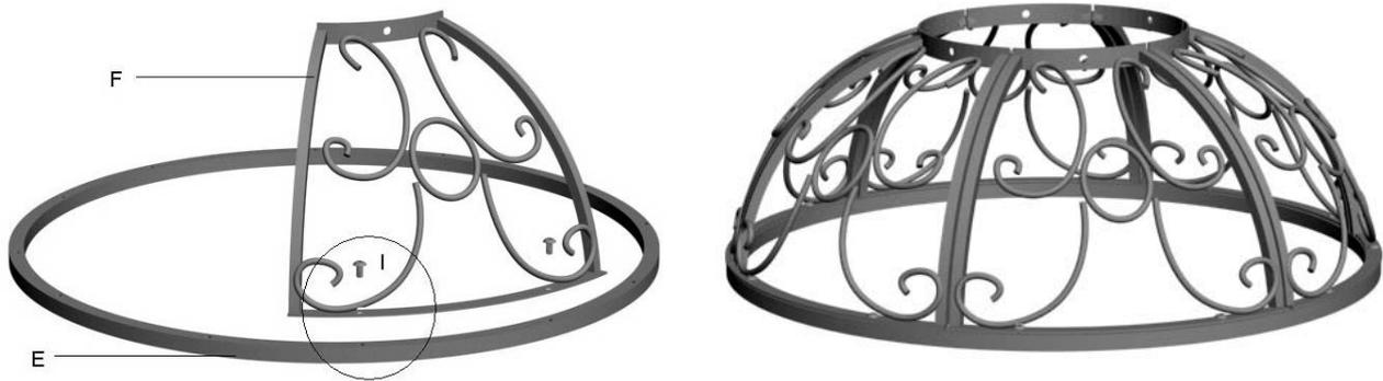
**Step 3:** Connect Base (G) to Decorative Frame (F) using Bolts (I) and Nut (J). Fully tighten all bolts.
