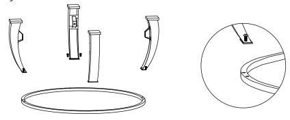
**Step 3:** Attach Lower Ring (H) to Legs (G) using M6 x 10mm Bolts (AA), tighten all the hardware.
