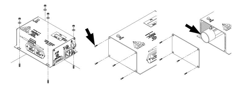
STEP 1) Disconnect all external connections. Remove the four screws from the Remove CO monitor from the unit.
