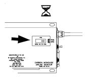
5. Adjust the "span" pot adjustment screw (clockwise to increase, counterclockwise to decrease) until the digital display reads the same concentration (ppm) as printed on the calibration gas cylinder.
