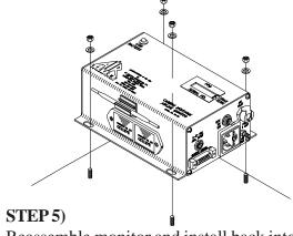
Reassemble monitor and install back into system. Connect all external connections. Allow monitor to stabilize 30 minutes to 1 hour and recalibrate.
