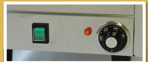
Covered master switch and adjustable thermostat
