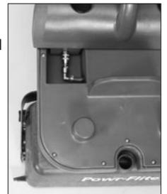
**IMPORTANT** – Only chemicals recommended by the manufacturer should be used, i.e. low foaming, and follow the chemical manufacturer's directions regarding use, handling, disposal and health and safety provisions. The tank capacity is 4 gallons. Do not overfill the tank as spillage may occur when in use.
