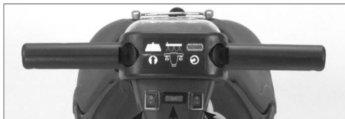
Vacuum motor switch    Neon indicator    Brush motor switch
