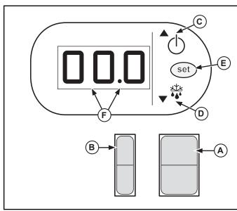
Figure 2. Heated Display Cabinet Switch and Panel .
