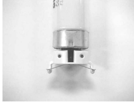
Bi-pin lamp end Properly installed lamp without shield. Verify identification mark identification mark is positioned as shown.
