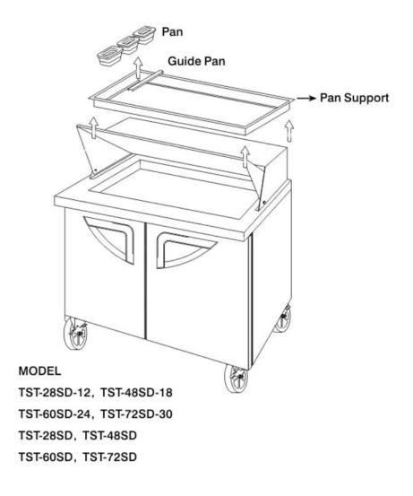
1) Remove the Guide Pans and Pans. Then pull out the Pan Supporter. Clean the pan supporter and reinstall in place.
