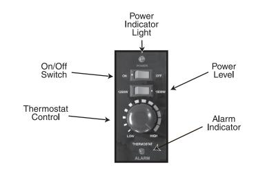
**POWER LEVEL SWITCH:** This heater has two heat settings: 1250 and 1500 watts. Use the higher setting (1500 WATT) to raise the room temperature quickly. When the desired temperature is reached use the lower 1250 WATT setting. It is usually sufficient to maintain a comfortable temperature.
