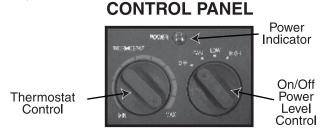
**POWER LEVEL SWITCH:** This heater has two heat settings: High and Low. Use the higher setting (1500 watt) to raise the room temperature quickly. When the desired temperature is reached use the Low setting. It is usually sufficient to maintain a comfortable temperature.
