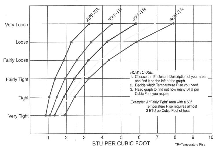
The heat requirement calculator provides general guidelines and is based upon a temperature rise from 20° - 60°F. On-the-job-site experience is a factor in final estimates. A job log is helpful for comparison of the estimates and final requirements, and further facilitates similar structure estimates.
