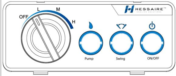
Rotary Switch/Motor Speed Has 4 positions. (Clockwise from OFF)
