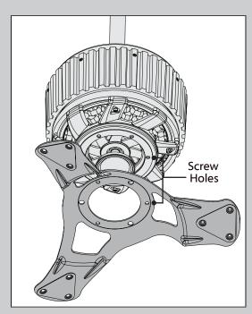
Lift a blade ring to the motor assembly and align the screw holes.
