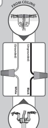
Using the orange wire connectors from the  $\bigstar$  hardware bag, connect the black wire (ungrounded) from the ceiling to the black wire from the fan. Connect the white wire (grounded) from the ceiling to the white wire from the fan.
