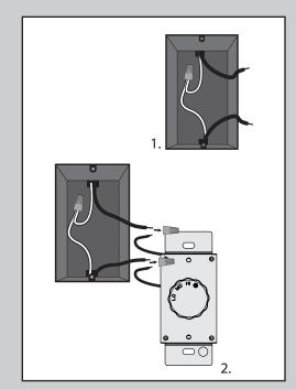
Using the wire connectors, connect each black wire from the wall control to a black wire from the switch box.
