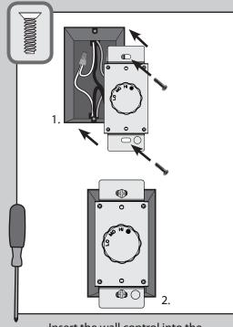
Insert the wall control into the outlet box and secure the two metal tabs to the tabs on the switch box using the two flat head screws that came with the switch box.
