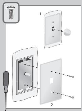
Remove the knob from the wall control and mount the faceplate (not included) to the wall control using the two #6-32 screws you removed earlier from the faceplate.
