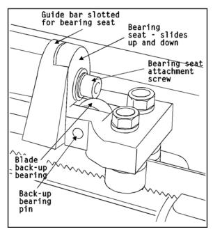
Figure 20: Adjusting back-up bearings
