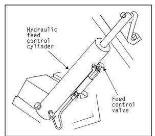
Figure 16: Hydraulic feed control
