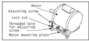
Figure 14: Motor plate adjustment screw
