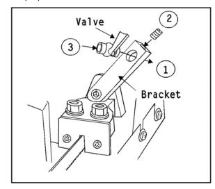
Figure 7: Installing valve in valve bracket
