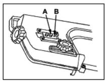
Figure 18: Blade tracking mechanism
