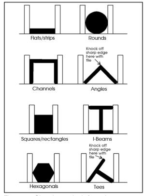
Figure 11: Clamping methods for various crosssections of stock
