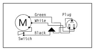
Figure 8: Wiring diagram
