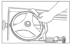
Figure 19: Checking blade tracking
