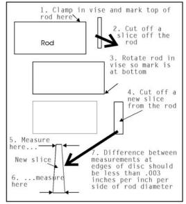
Figure 22: Making a test disc.
