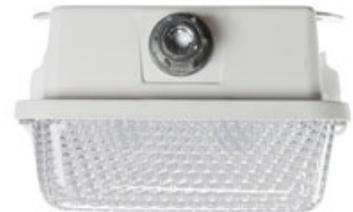
This Class 1 Division 2 rated fixture is constructed of non-corrosive materials including a polyester housing reinforced with glass fiber, a poured in gasket for reliable sealing and an impact resistant acrylic diffuser. Eight corrosion resistant plastic latches secure the lamp cover to the housing and provide a firm lock against the poured in seal to prevent drips and water intrusion.
