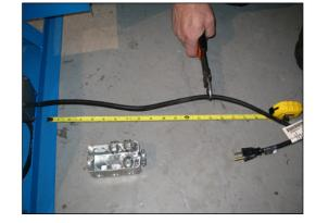
Step 3: Cut existing motor power cord 14" from motor.
