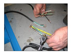
Step 4: Remove 4" of insulation from cut ends and enclosure safety switch cord.
