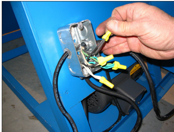
Step 9: Connect wires per schematic. Connect all four ground wires and attach mechanically to box per code. Wire nut all connections.
