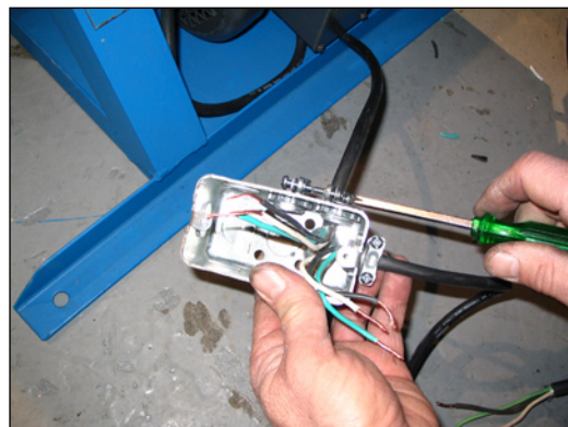
Step 6: Install motor wire through the lowest side hole. Tighten screws.
