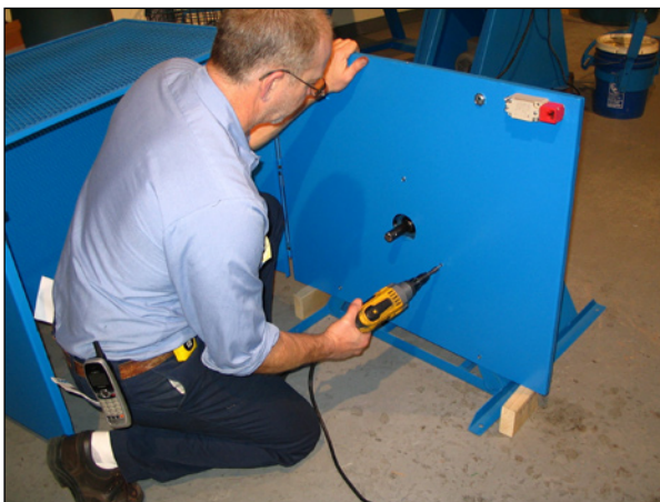
Step 8: Screw 5 self drilling screws through back panel and into the angle frame.
