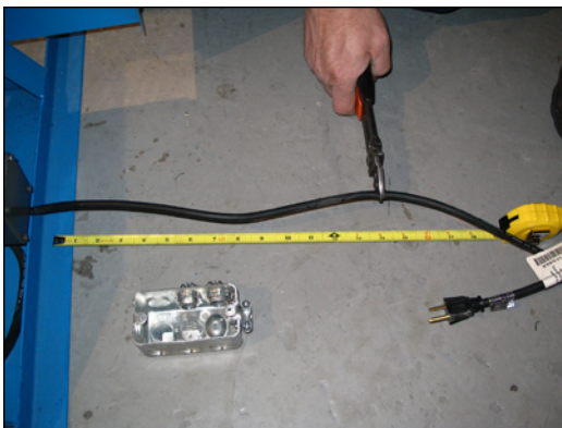
Step 3: Cut existing motor power cord 14" from motor.
