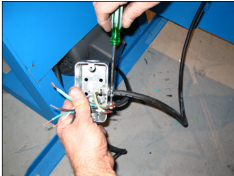
Step 7: Install safety switch wires through the middle side holes. Tighten screws.
