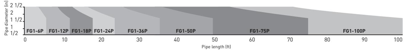
Add 1 foot to your pipe length for each valve or spigot on your pipe system. If cable selected is longer than the pipe, spiral it evenly along the entire pipe.
