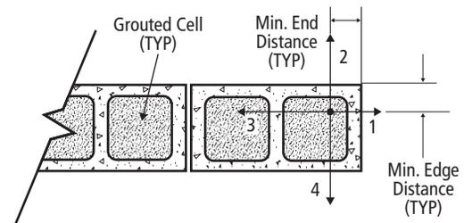
1. Shear load parallel to Edge and perpendicular to End
