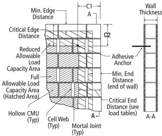
**Direction of Shear Loading in Relation to Edge and End of Masonry Wall**
