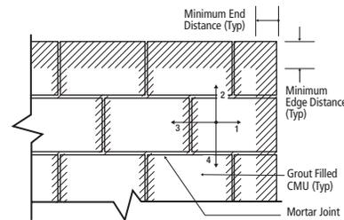
1. Shear load parallel to Edge and perpendicular to End
