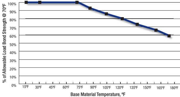
**Load-Temperature Reduction Curve
