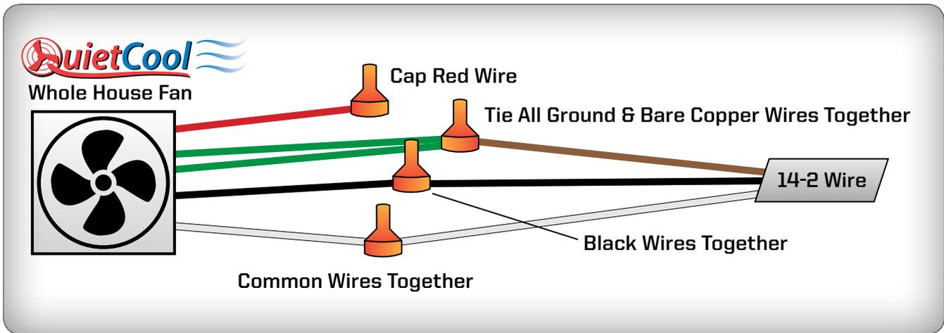
6. Start by wiring the first motor head. Open up the handy box and take off all the wire nuts. Unscrew the green ground wire and detach the green ground wire from the power cord. Remove the power cord. Reattach the green ground wire to the handy box. Cut your green ground wire in half and strip both sides.
