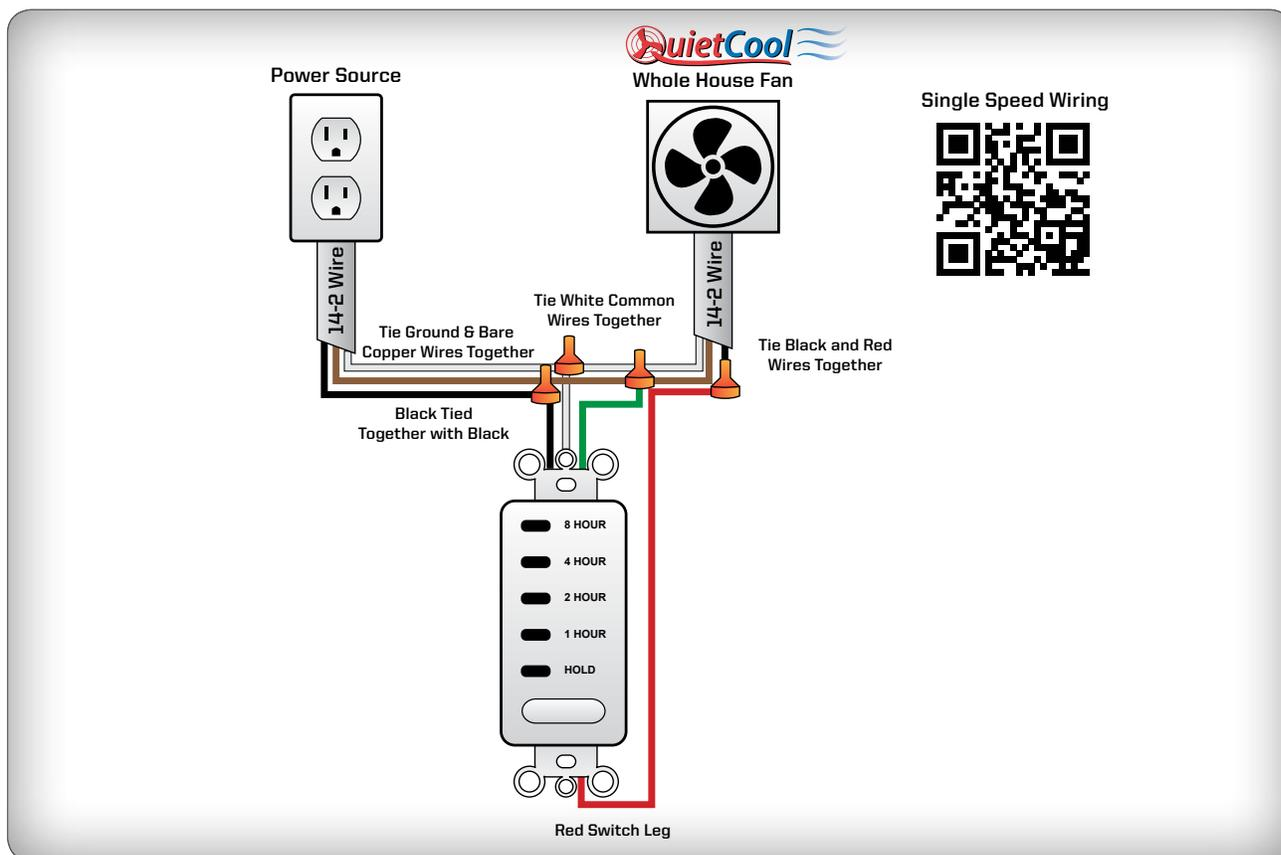
2. Using a wire nut, tie the black wire on the 2 wire Romex from the fan to the red wire on the timer.
