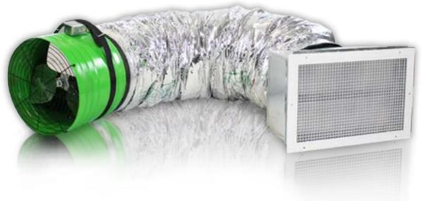
6. Hang the motor head from the rafters by fastening the metal strapping that is attached to the motor head to the rafters with the wood screws. Make sure the power box on the motor head is at the very top. Secure duct to damper box using three black sharp screws. Make sure the duct has a gentle 90 degree bend to help reduce noise level.
