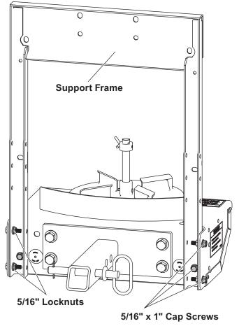
3. Mount the throat support to the support frame at the two lower holes by using the four supplied 5/16" x 1" cap screws and 5/16" locknuts. Tighten the fasteners according to the torque chart.
