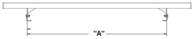
"A" spacing is to the outside edges of the mounting feet before attaching the curved mounting plates.
