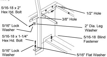
STEP 8. Tightening fasteners.
