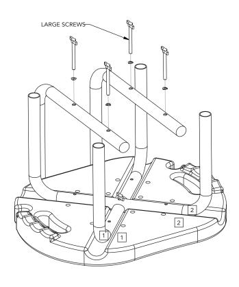
Place L bar over U bar holes so holes line up. Screw in using long screws - include washer. Do not tighten yet.
