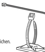
Use cable ties and clips to bundle cables where needed.
