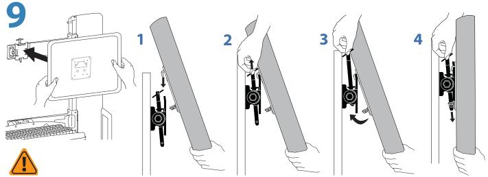
**WARNING:** The monitor will not be securely attached until the Locking Pin passes through the tab on the Quick Release Bracket. Do not leave the monitor unsupported until you are certain the Locking Pin is in place.
