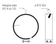
Fold out the tabs as shown using needlenose pliers. 2. Hang the fan using suitable hardware.
