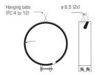
Fold out the tabs as shown using needlenose pliers. Hang the fan using suitable hardware.
