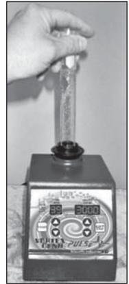
To initiate the PULSE “ON” mode, press the **PULSE** button until **ON** is illuminated beneath the word **PULSE**. The **TIME** and **SPEED** displays will begin flashing. When display is flashing, you are setting the Pulse “RUN” time (left display) and the Pulse “STOP” time (right display).
