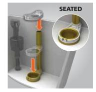
**Step 13**: Slide the BRASS SEAT ADAPTER down the pipe and snap it to the FLUSH VALVE SEAT as shown.
