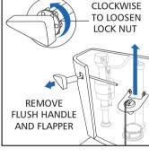
**Step 3**: Remove the existing flapper, chain and flush handle assembly from your tank. When removing the FLUSH HANDLE, note that the LOCK NUT may be reverse-threaded, so you need to turn it clockwise to loosen it.
