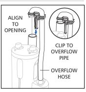
**Step 19**: Attach the OVERFLOW HOSE to the top of the OVERFLOW PIPE via the black plastic OVERFLOW HOSE CLIP. Ensure that the opening of the OVERFLOW HOSE is directly aligned with the opening of the OVERFLOW PIPE.
