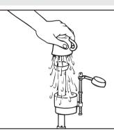
**Step 2**: FLUSHING OUT DEBRIS: Hold a cup over the uncapped valve to prevent splashing. Turn water supply full on and off a few times. Leave water supply off.
