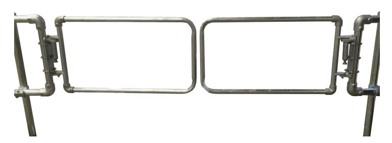
When an opening is larger than what a single gate would typically accommodate the Kee Safety Double Gate provides an ideal solution, easily able to span openings between 3 and 6 feet across. The gate can be modified on-site to suit the exact opening and is supplied with a simple screw adjustment to ensure precise alignment where both gates meet.
