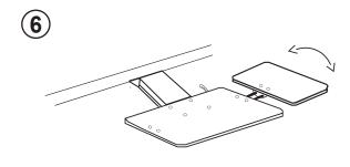
6. Press down to tilt the Mouse Pad and adjust its' angle. If the mouse pad is too loose, tighten the 2 screws on the mouse pad mounting bracket.
