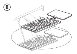
8. KTI is adjustable in height and angle. Release the lever (7A), adjust to your desired position, and lock the lever in place.
