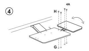
4. Connect the metal Mouse Pad Bracket to the keyboard tray using 2 H Screws & 2 G Nuts. 4A. Connect the Mouse Pad to the Mouse Pad Bracket using 2 H Screws & 2 G Nuts.
