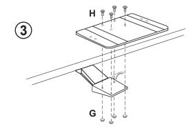
3. Attach the Keyboard Panel (C) to the mounting panel with 4 H Screws & 4 G nuts.
