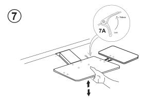
7. The Keyboard Tray slides in/out by pushing/pulling. 7A. To adjust the Keyboard Tray's angle, release the lever under the keyboard tray.
