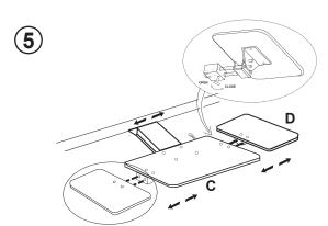
5. The Mouse Pad (D) attaches to the right or left side of the Keyboard Tray (C). Release the thumb screw on the attachment to move the Mouse Pad closer to or farther away from the Keyboard tray.
