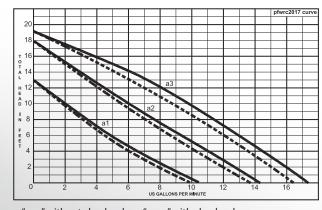
"\_\_\_" without check valve, "\_\_\_" with check valve
