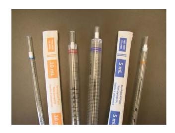
SCILOGEX disposable Serological Pipets are manufactured from optically clear polystyrene in a class 100,000 clean room. The 1ml, 2ml and 5ml are a one piece construction and the 10ml, 25ml and 50ml pipets are made with a durable ultrasonically welded 3 piece construction.
