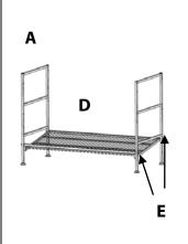
**2.** Using four SCREWS (E) and the HEX KEY (F) loosely secure the bottom SHELF (D) to each side frame. Once all the screws are in place, tighten down all the screws.
