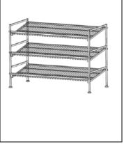
**3.** Once all shelves are securely in place, adjust the leveling feet by screwing them in or out to obtain a level rack.
