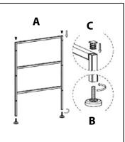
**1.** Screw the LEVELING FEET (B) into the legs of each SIDE FRAME (A). Insert the CAPS (C) into the top holes of each side frame.
