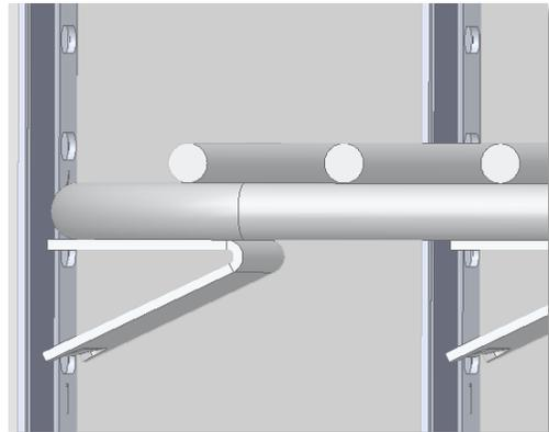
Figure 7: SRI3P Shelf Installed
