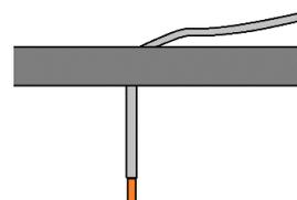
**Figure 18: Probe End 2 inches (5cm) From Shelf Surface**
