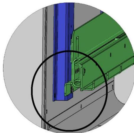
**Figure 14: Sliding Mounting Bracket Front Screw Installed**
