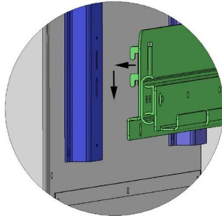
**Figure 13: Sliding Shelf Mounting Bracket Installation**
