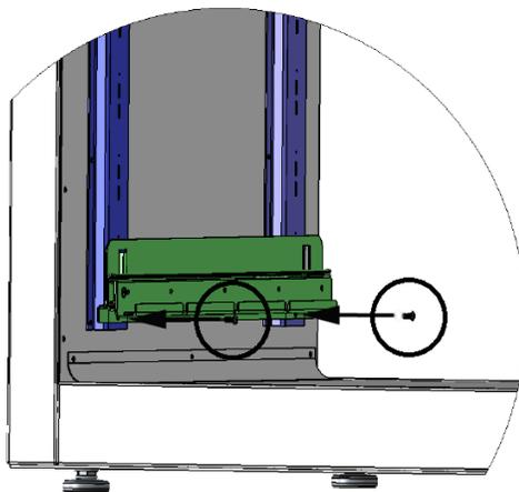
**Figure 15: Sliding Mounting Bracket Screws**
