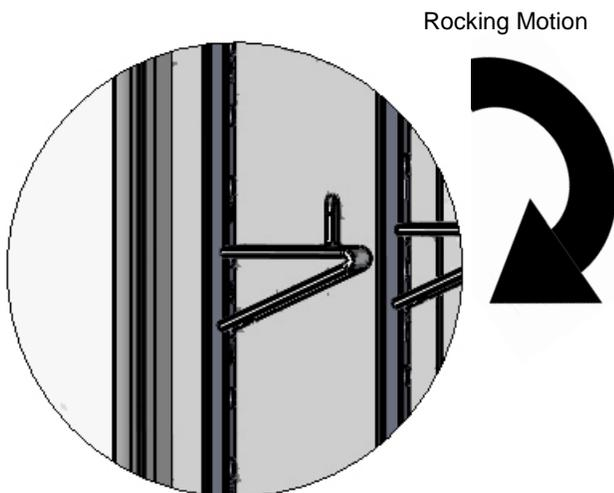
Figure 8: SRI3P Shelf Clip Installed
