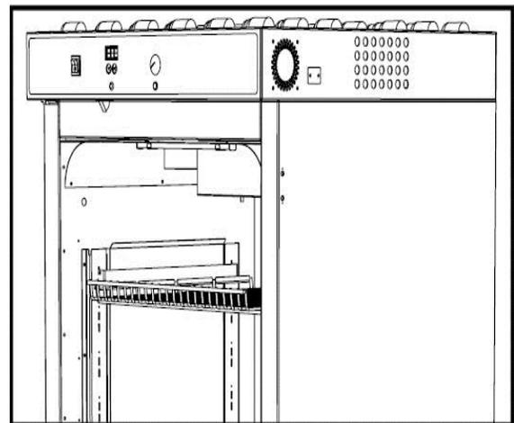
**Figure 11: Standard Shelf Installed**
