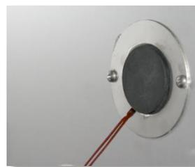
Figure 17: Introducing a sensor probe through the access port.
