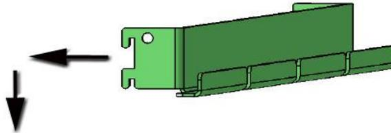
**Figure 9: Standard Shelf Mounting Bracket Installation**
