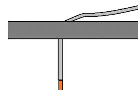
**Figure 20: Probe End 2 inches (5cm) From Shelf Surface**
