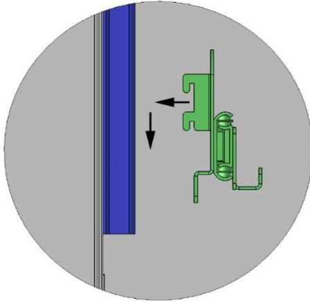
**Figure 12: Sliding Shelf Mounting Bracket Installation**
