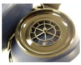
Check and replace worn or damaged parts. Pay special attention to the exhalation membranes. Making sure that they are clean and intact is as important as regular filter replacement.
