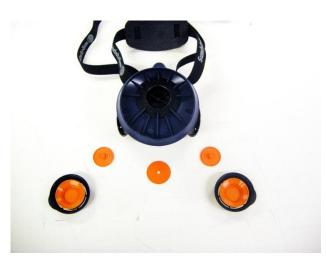
Remove the filter and the membranes. Clean the mask with the Sundström antibacterial cleaning tissue SR 5226.
