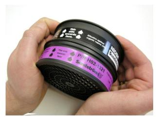
Press the filter/cartridge together so that the arrows on the particulate filter point towards the chemical cartridge.
