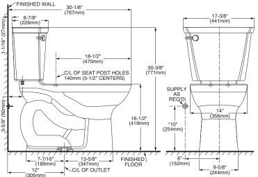
THIS TOILET IS DESIGNED TO ROUGH-IN AT A MINIMUM DIMENSION OF
