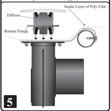
Once diffuser is seated flush against the bracket rotate the diffuser clockwise 60° to lock the diffuser to the bracket.
