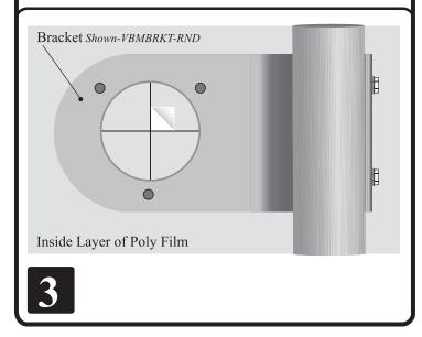
Attach the shaded pole blower to the bracket as shown. The configuration and number of threaded pins is dependant on the model of bracket. The VBMBRKT-SQ will have 4 threaded pins in a rectangular formation and will require the use of 4 lock nuts to fully secure the blower. The VBMBRKT-RND will have 3 threaded pins in a triangular formation and will require the use of 3 lock nuts to fully secure the blower motor.
