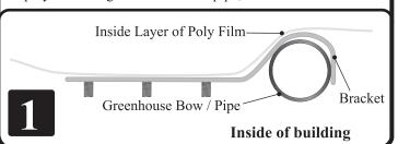
Observe the two sets of predrilled holes in bracket on curved end of bracket. Choose the set that best aligns with the greenhouse bow / pipe center. Secure bracket to greenhouse bow / pipe using 2 included self tapping TEK screws.
