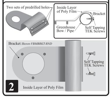
Using the vent hole in the bracket, cut a + in the inside layer of poly film, making sure not to exceed the vent hole opening. Do NOT cut a round hole.
