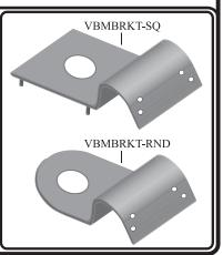
Insert bracket with curved area placed BETWEEN inside layer of poly film and greenhouse bow / pipe, as shown below.
