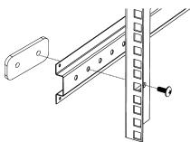
Unscrew the rail from the rail support. Move the rail forwards or backwards to desired location. Insert screw and secure.
