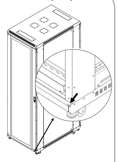
Remove the plastic bushing from the bottom pan of keyed side. This is inserted to help support the door during shipping, but is not needed once the cabinet is installed.
