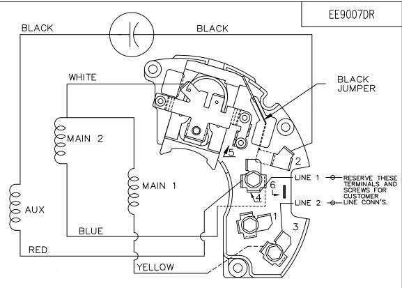
SINGLE HIGH VOLTAGE CAPACITOR START REVERSIBLE ON TERM BOARD NO OVERLOAD PROTECTION
