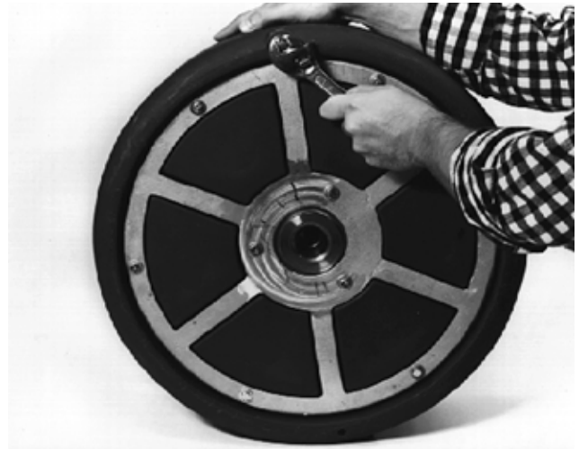
Figure 23 – Removing Pigtail Anchoring Bolt
