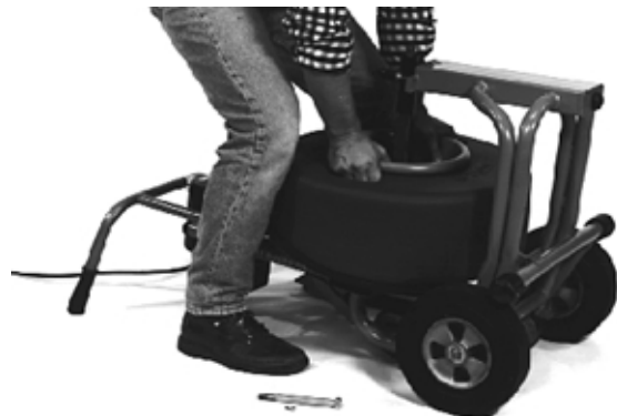
Figure 20 – Lifting Drum Assembly Onto Frame
