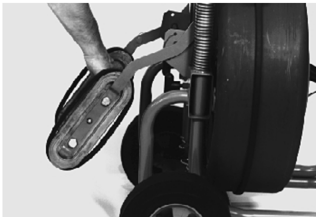
Figure 3 – Relevage du monte-marches
