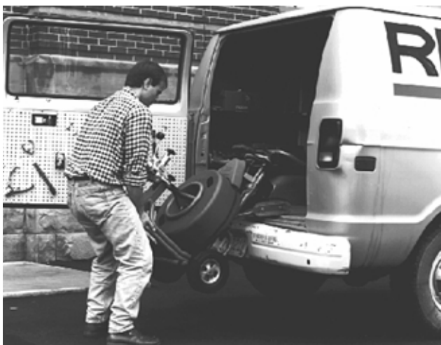
Figure 12 – Lifting Unit Onto Vehicle
