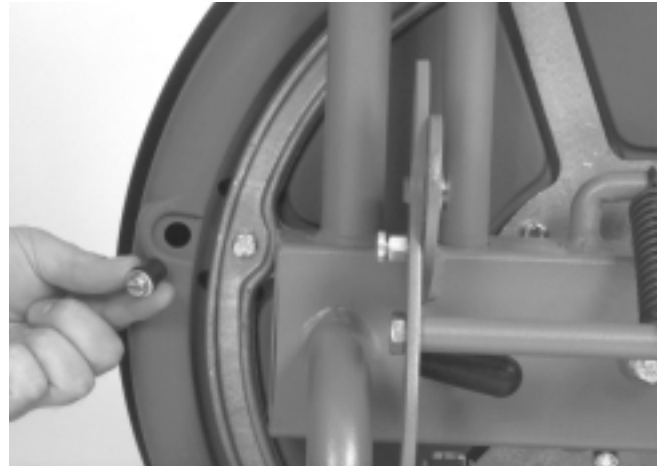
Figure 13 – Drum Drain Hole
