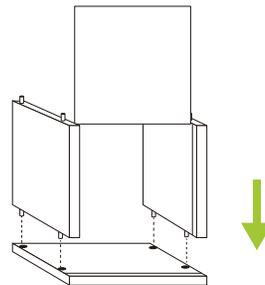
**3** Align vertical zBoards and backer board to horizontal zBoard.
