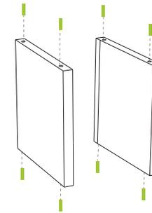
**2** Place alignment pins in vertical zBoards.
