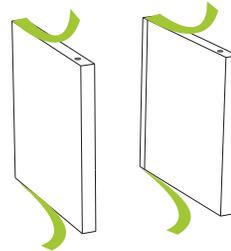
**1** Carefully remove the 3M protective layer from adhesive.
