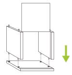
Align vertical zBoards and backer board to horizontal zBoard.
