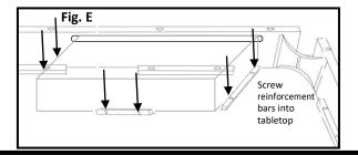
**CAUTION:** Double check all screws to be tightened securely before use. Check all screws periodically.
