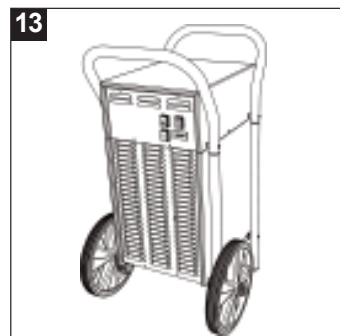
13 Position unit upright. Wait 30 minutes before starting to allow compressor to drain back.
