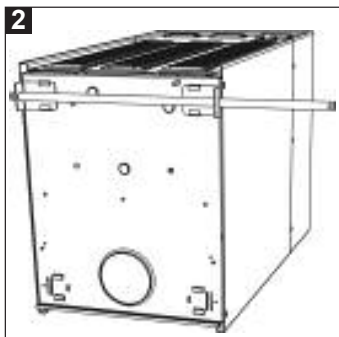
2 Slide wheel axle into wheels brackets. Offset to one side.
